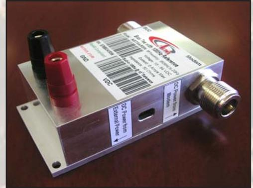
This small and efficient unit provides 10MHz high stability ( $10^{-8}$ ) reference and DC supply to a BUC in case a modem neither cannot supply sufficient power nor 10MHz reference. The unit passes L-Band signal and injects 10MHz reference signal or up to 6A DC current.
